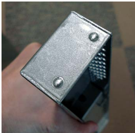
Fig. 2 - Bumps on right end of bezel
