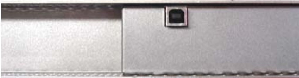
Fig. 4 - Section of back of bezel with USB B-type plug
