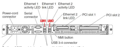
Portion of 505 model chassis rear with LAN ports identified
