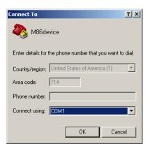
C. At the **Connect using** field, select the COM port assigned to the serial port on the laptop (probably "COM1"), and then click **OK** to open the Properties dialog box, displaying the Port Settings tab:
