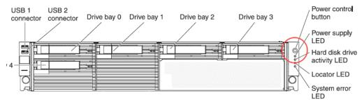
Fig. 10 - 705 / 735 model front panel, power button at far right
