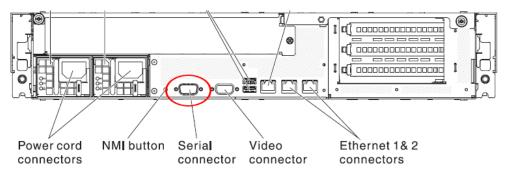
Fig. 5 - Rear of 705 / 735 model chassis, serial port circled in red
