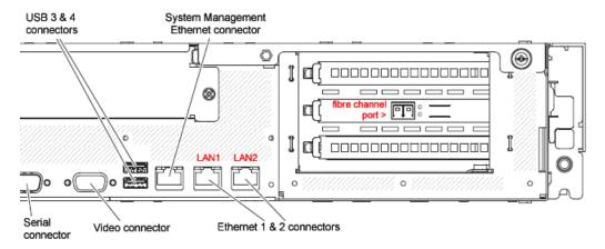
Figure 2: Diagram showing right portion of SR 735 chassis rear
