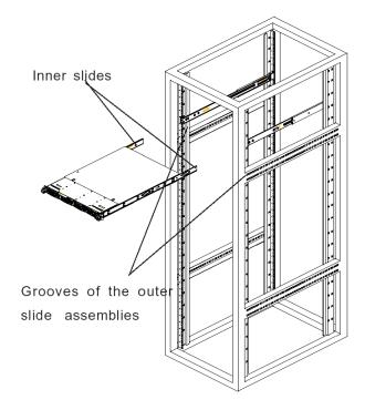
2. Push the chassis all the way to the back of the outer slide assemblies as shown below:
