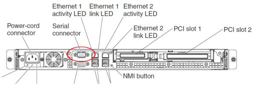
Fig. 4 - Rear of 505 model chassis, serial port circled in red
