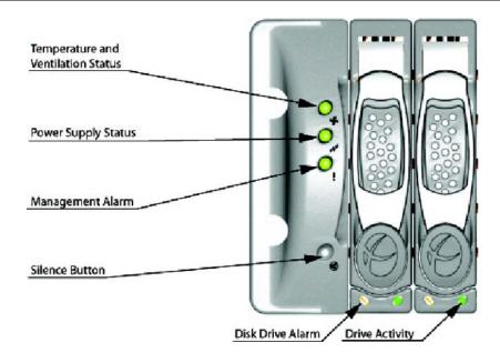
When the LED is green, the blowers are operating at an acceptable RPM, and the internal temperature sensors are within acceptable limits.
