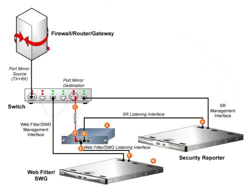
Diagram showing Ethernet Tap installation on the network
