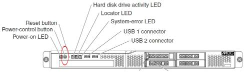
Fig. 9 - 505 model front panel, power button at far left
