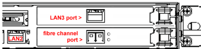
Figure 1: Diagram showing right portion of SR chassis rear
