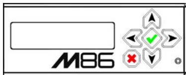
Fig. 4 - 300 series LCD panel and keypad
