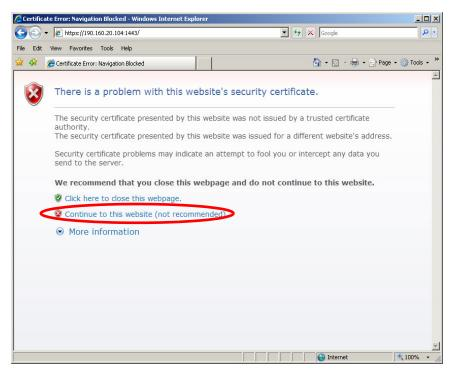
Selecting this option displays the SR login page with the address field and the Certificate Error button to the right of the field shaded a reddish color:
