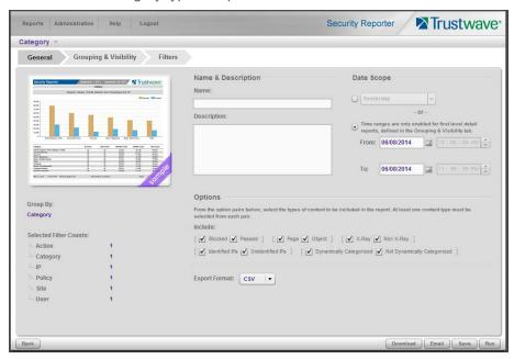
The Report Wizard is comprised of three tabs used for specifying reporting criteria: General, Grouping & Visibility, and Filters. The bottom right of the panel includes the Download, Email, Save, and Run buttons.
