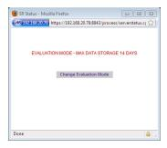
Until the SR is in registered mode, this pop-up box will continue to open whenever accessing the System Status screen of the System Configuration administrator console.
