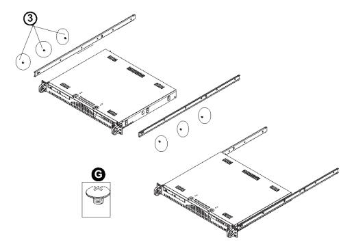
4. Attach an inner rail to each side of the chassis and secure the inner rail to the chassis by inserting three Type G screws through the holes on each side of the chassis and the inner rail. (See the diagram below for a description of the Type G screw.)
