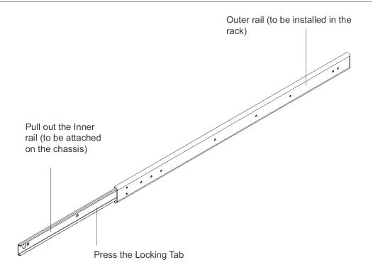
3. Locate the three holes on each side of the chassis and locate the three corresponding holes on each of the inner rail.
