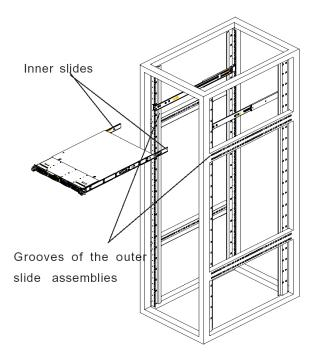
2. Push the chassis all the way to the back of the outer slide assemblies as shown below:
