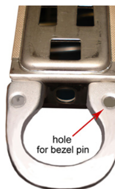
Inside front end of U-shaped handle on left inner rail
