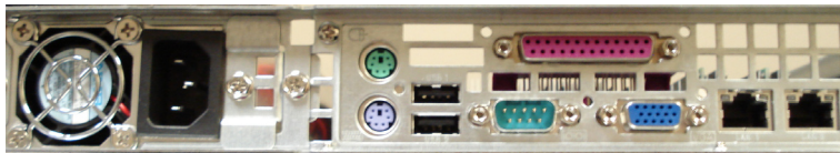
Rear of the chassis
