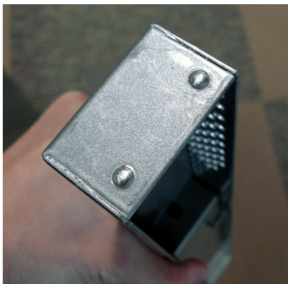
Fig. 2 - Bumps on right end of bezel
