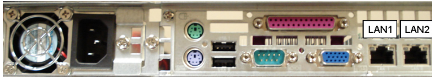
Fig. 1 - Portion of SL and MSA chassis rear
