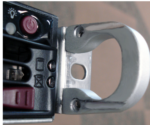
Fig. 3 - Grooves in right U-shaped handle
