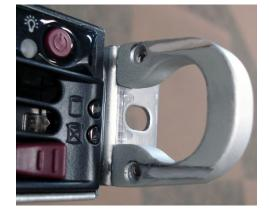
Fig. 2 - Bumps on right end of bezel
