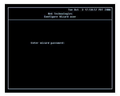
C. At the **Enter wizard password** field, enter the password that will be used to access the setup wizard in the Threat Analysis Reporter interface. Press **Y** for "Yes" to confirm and save your entry and to go to the Quick Start Setup confirmation screen.
