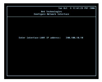
A. At the **Enter interface lan1 IP address** field, enter the IP address for the LAN 1 interface, and then press **Enter** to go to the next screen.
