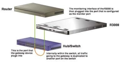
Fig. 1:1-2 Invisible mode diagram, with port monitoring
