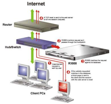
Fig. 1:1-1 Pass-by filtering diagram
