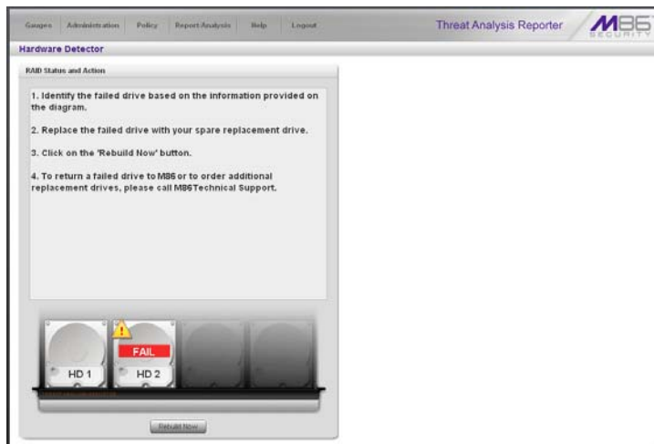
Fig. C-1 Hardware Detector panel, failed hard drive detected
