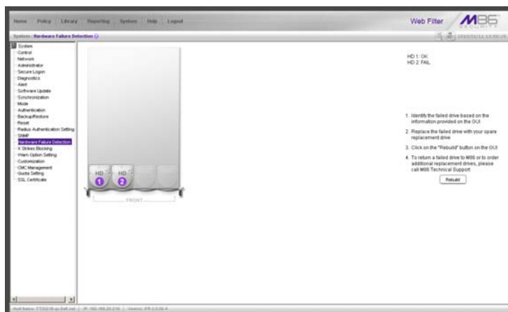
Fig. 2:1-62 Hardware Failure Detection window, 500 and 700 series
