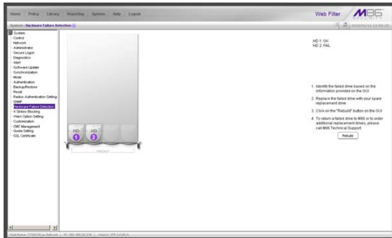
Fig. F-2 Hardware Failure Detection window, 500 and 700 series
